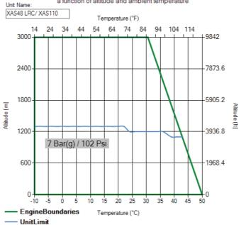
Graph represents working conditions, for starting conditions pls contact your Atlas Copco contact
